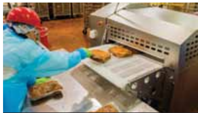
The 5-pound pouches of barbacoa beef run through a flattener that helps pre-shrink the package for the restaurant.
